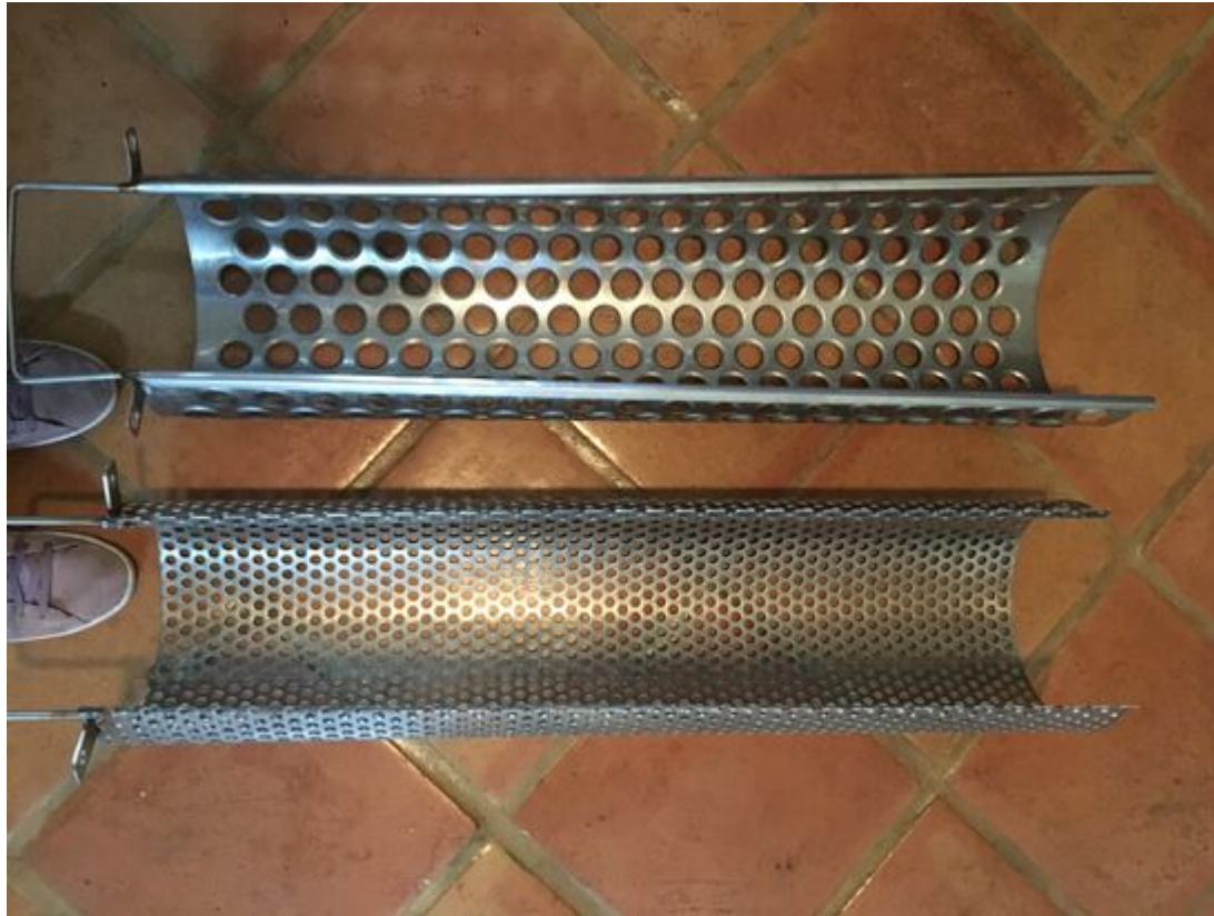
Original destemmer basket above, modified basket below. Make sure to keep the handles, tabs for securing, and also the RAILS that go along each edge
